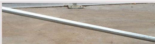
1.315in Round Tubing used as Support Rail
