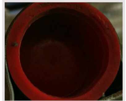
Round Cap Plugs used for Both Ends of Round Tubing Support Rails
