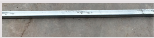
1 1/4in Square Tubing used for Leg Support Crossbars
