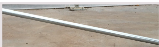
1.315in Round Tubing used as Support Rail and Standard Rollers
