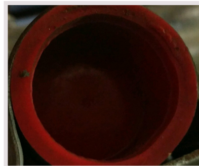
Round Cap Plugs used for Both Ends of Round Tubing Support Rails and Standard Rollers
